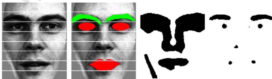
Fig. 8. Left to Right: One of five training images. Test image showing marked saliency. Saliency predictions using KNC with 11 centroids. Saliency predictions using 1000 random forest trees per partition.
