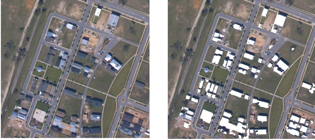
Figure 3. An image from coastal florida (left). Extracted buildings are shown in white (right).
