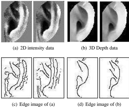
**Figure 3. Same ear’s 2D and 3D Ear Data and Associated Edge Images. Canny Edge Detector Parameters are  $\sigma = 1.0$ ,  $T_{low} = 0.5$ ,  $T_{high} = 0.5$**
