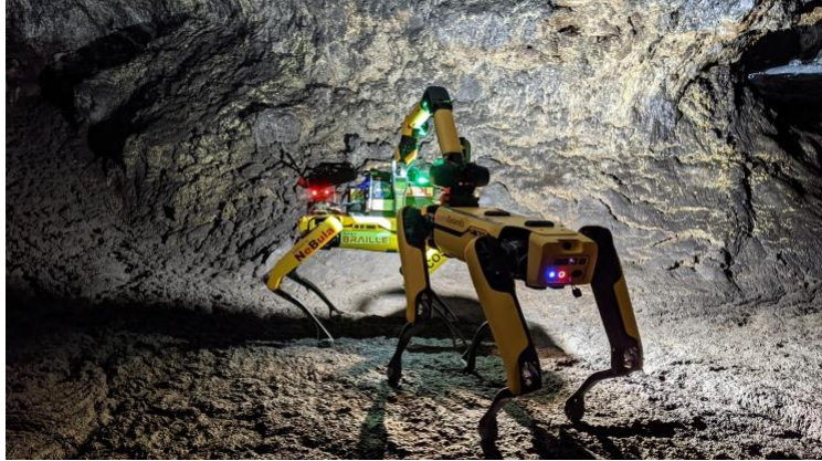
Figure 1.1. Two Nebula-SPOT quadruped robots developed by Boston Dynamics and deployed by NASA to explore a cave as part of the Defense Advanced Research Projects Agency Subterranean Challenge. Engineers at the Jet Propulsion Laboratory equipped the quadruped with sensors and autonomy software to enable it to construct maps of underground cave systems and urban environments. In the future, these robots may be deployed to map and explore cave systems on other worlds, potentially to collect scientific samples in search for signs of alien life.
