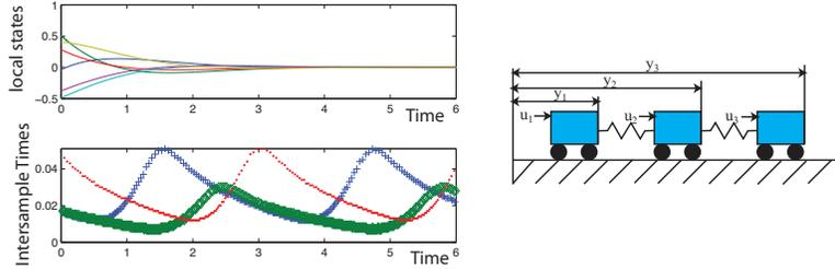
Figure 2: Simulation Example of Event-Triggered Networked Control System consisting of three coupled carts.
