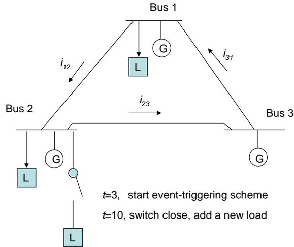
Figure 4.6. Three generator simulation model
