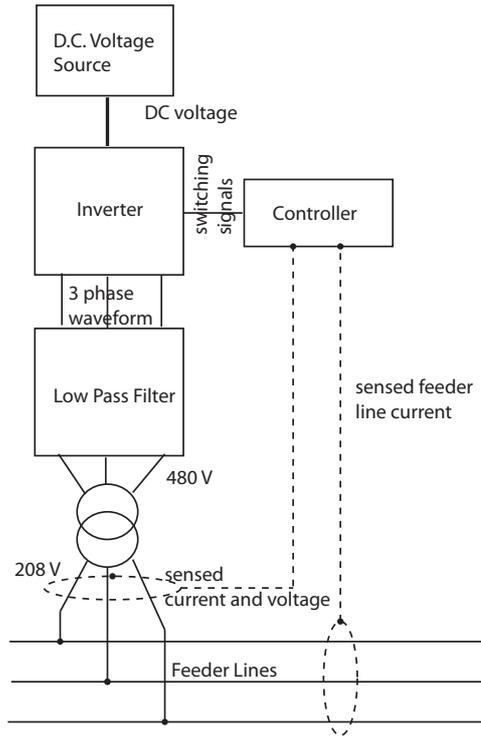
Figure 4.2. Inverter-based microsource
