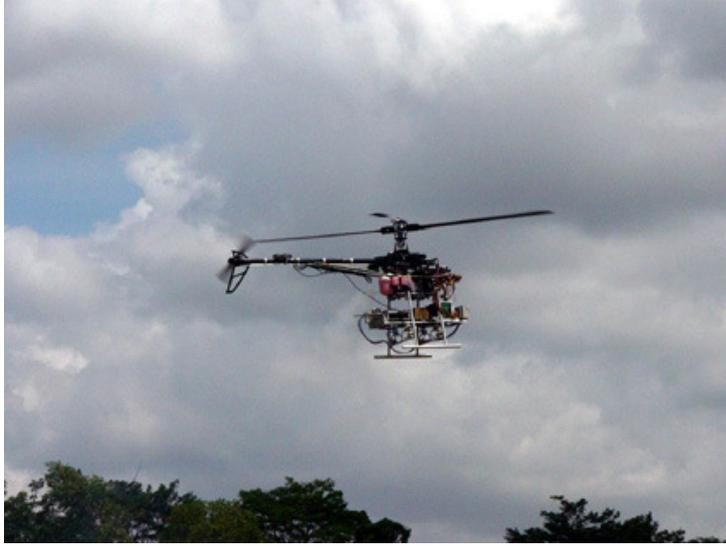
Figure 1. An Autonomous UAV Helicopter.
