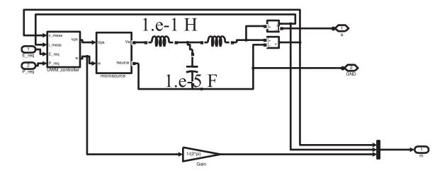
• Large inductors (1.e-1 H) needed to be used in the simulation to prevent simulation breaking down. (Is this an issue related to scale of the sources?)
