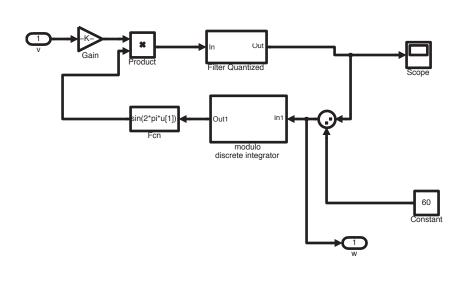
Phase-locked loop (60 Hz)
