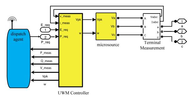
Figure 2 identifies the signals within the UWM controller are required by the dispatch agent. This figure shows the simulink block diagram for the UWM controller. The signals to be passed over the interface are
