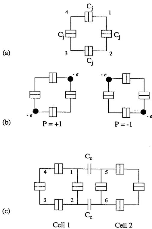
FIG. 1. (a) The ring of tunnel junctions that forms a basic cell. (b) Coulomb effects tend to localize the two extra electrons in one of the two configurations shown. These have polarization of  $+1$  and  $-1$ . (c) Two capacitively coupled cells.
