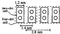
Fig. 2. Cell to cell distance of a four dot QCA cell built from two 2-dot molecules.
