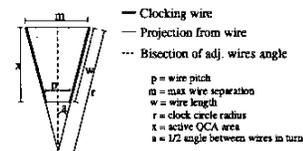
Fig. 5. Parameters used to calculate clocking wire density on a turn for the perpendicular clocking wire layout.
