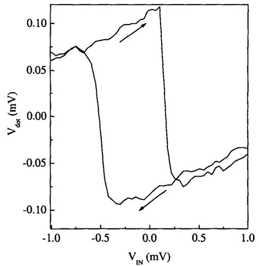
Figure 3. Demonstration of the "memory" in the clocked QCA cell
