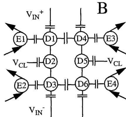
Figure 1. (A) SEM micrograph of the clocked QCA cell (B) Schematic diagram of the device
