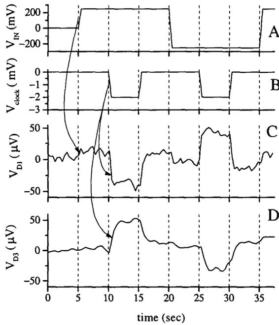
Figure 2. Clocked QCA cell experiment. From top to bottom: (A) signal input; (B) clock input; (C) signal measured on dot D1; (D) signal measured on dot D4.
