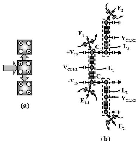
**Figure 1.** Schematic of a QCA fanout gate: (a) using full QCA cells and (b) a metal-dot based implementation consisting of three QCA latches. Individual latches are delineated with dashed lines.
