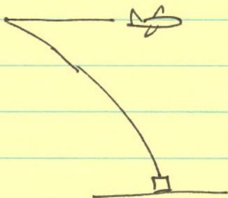
Horizontal velocity of plane & crate remains the same, so crate fall vertically down wrt plane.
