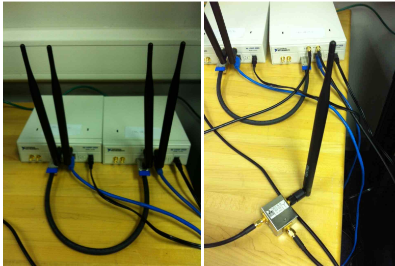
(a) Hardware setup with two antennas (b) Hardware setup with one antenna and circulator
