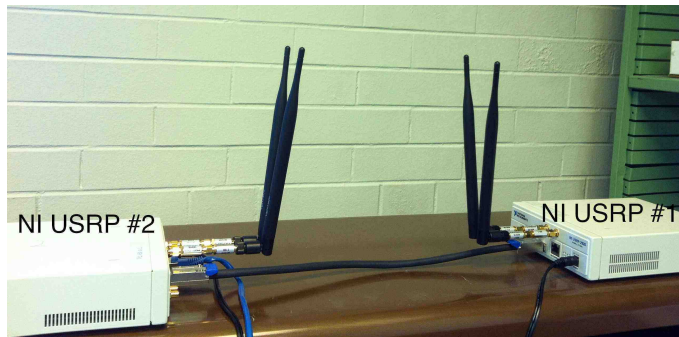
(b) Bidirectional setup with two antennas
