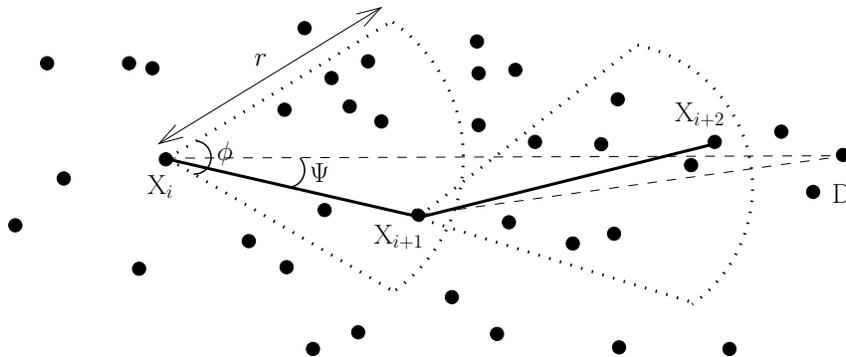
Fig. 5. The greedy forwarding strategy. Each relay  $X_i$  forwards the packet to its farthest neighbor lying inside the sector of radius  $\phi$  around the  $X_i$ -D axis. The thick lines represent the path taken by the packet (through three arbitrary relays) for this particular realization.
