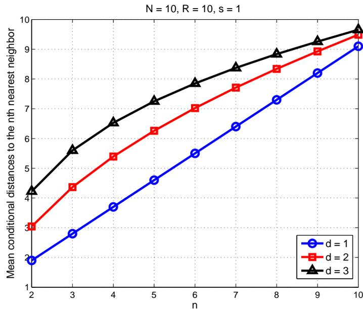
Fig. 7. The mean conditional distances of the higher-order neighbors in a binomial network with 10 nodes and  $d = 1, 2, 3$ , when it is known that the nearest neighbor is at unit distance away from the base station.
