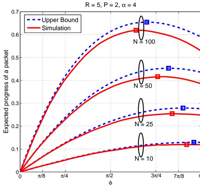
Fig. 6. The expected progress of a packet (empirical and upper bound) for various values of  $N$ . The square markers correspond to the optimum values of  $\phi$  that maximize the packet's progress.
