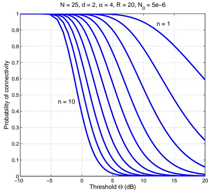
Fig. 9. The probability of the  $n^{\text{th}}$  nearest neighbor,  $n = 1, 2, \dots, 10$ , being connected to the BS for a binomial network with 25 nodes.
