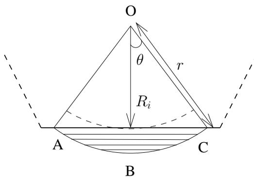
Fig. 3. Section of a  $l$ -sided regular polygon depicting one of its sides.  $O$  is the origin. For  $R_i < r \leq R_c$ , the area of the shaded segment  $ABC$  is  $r^2\theta - R_i\sqrt{r^2 - R_i^2}$ .
