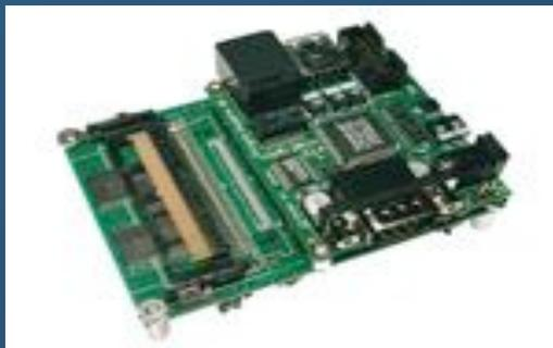
Stargate: bridges a sensor network of Berkeley motes to an 802.11 network
