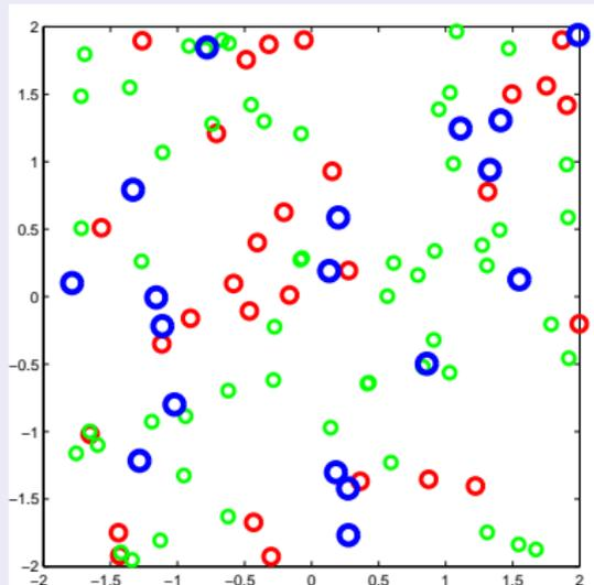
Base stations in each tier form independent Poisson point processes (PPPs) of densities  $\lambda_i$  and transmit powers  $P_i$ .
