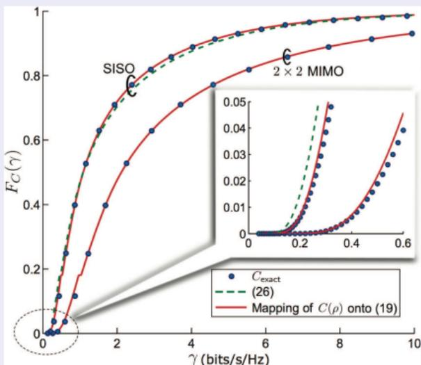
With SISO, essentially no user gets less than 0.18 bps/Hz. With  $2 \times 2$  MIMO, no user gets less than 0.3 bps/Hz.
