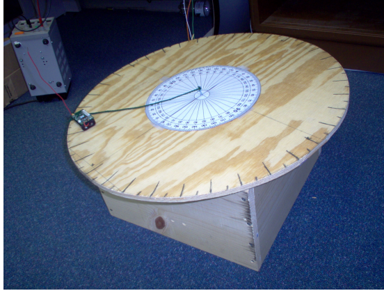
Figure 2.2. Turntable used for experiments verifying spatial diversity.
