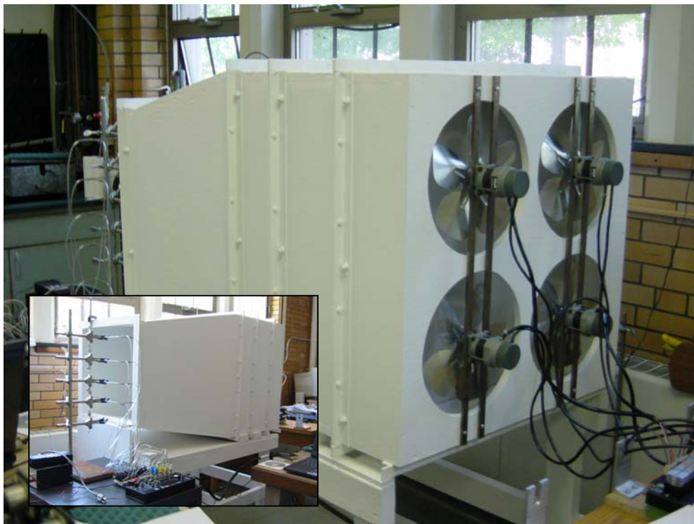
Figure 2: Transient Flow Field Simulator (TFFS) at the NatHaz Laboratory
