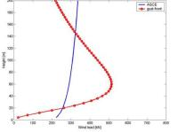
Figure 2. ESWL in ASCE 7 and gust-front wind
