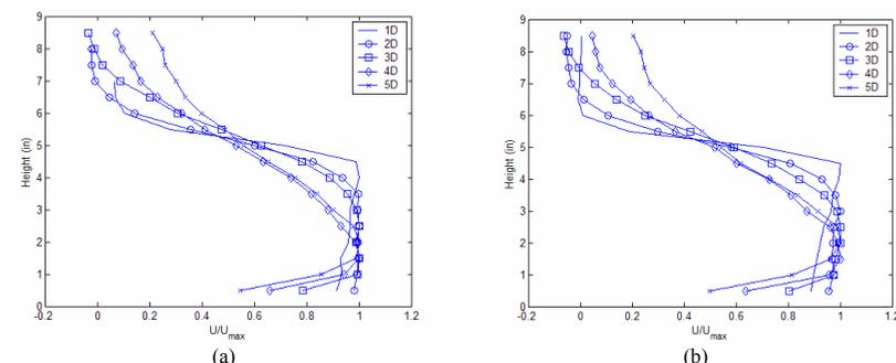
Figure 2: Profile development beyond a flat plate at (a) 45° incidence and (b) 50° incidence.
