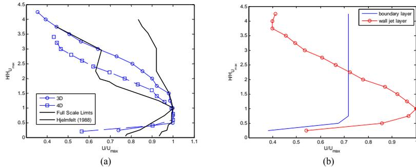
Figure 3: (a) Profile development beyond a flat plate at 30° incidence and (b) boundary layer profile comparison during simulated storm event (4D with the flap at 30° incidence).
