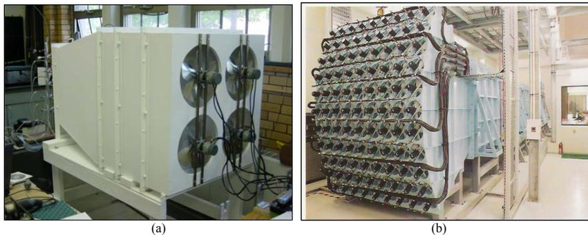
Figure 6: (a) The prototype transient flow field simulator and (b) multiple fan wind tunnel at Miyazaki University.
