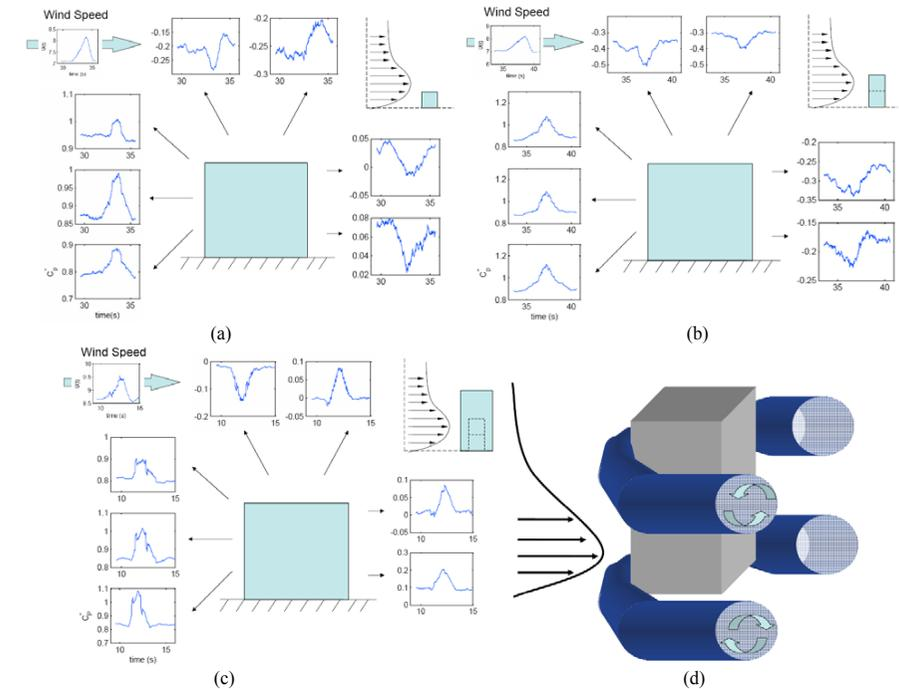
Figure 4: Pressure coefficients on a prismatic model of aspect ratio (a) 1:1 (b) 2:1 and (c) 2:1x2 during a simulated gust front event, and (d) a caricature of the flow development around a prismatic model.
