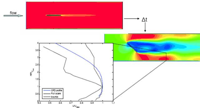
Figure 5: CFD model of the flat plate experiment utilizing a dynamic mesh to model the plate movement and an examination of the wind speed profile compared with full scale data.
