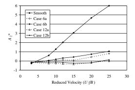
Figure 4 Flutter derivative  $A_2^*$  in smooth and turbulent flow.
