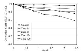
Figure 10 Cross correlation coefficients ( $\tau = 0$ ) for total lift with the model oscillating at  $U_r = 20$ .
