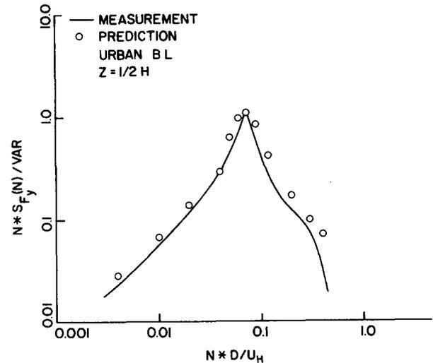
Figure 1 Predicted and measured normalized reduced spectra of acrosswind force
