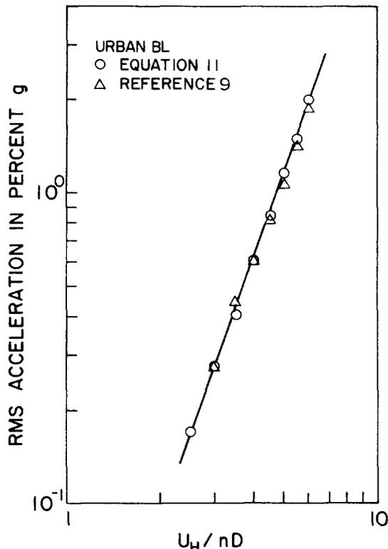
Figure 8 Comparison of predicted rms acceleration response
