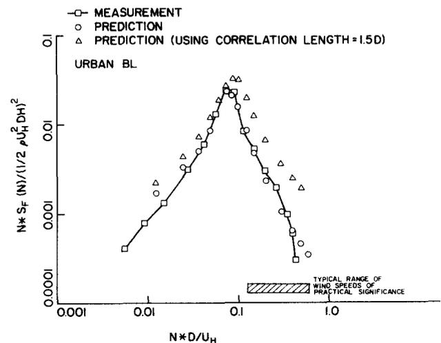
Figure 5 Predicted and measured mode-generalized spectra for urban flow
