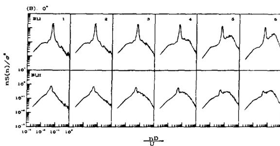
Fig. 5: Pressure Spectra on Side Face
