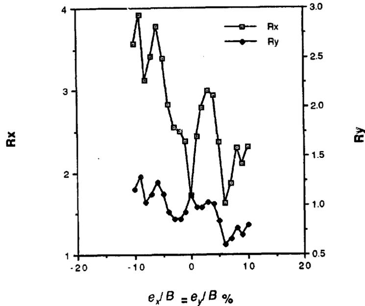
Figure 4. Influence of eccentricity between mass and elastic centers on the building response.
