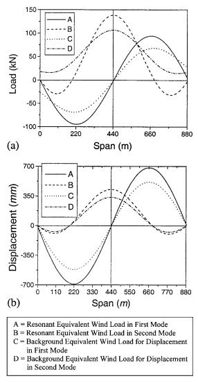
FIG. 2. Wind Loading and Effects on Humen Bridge
