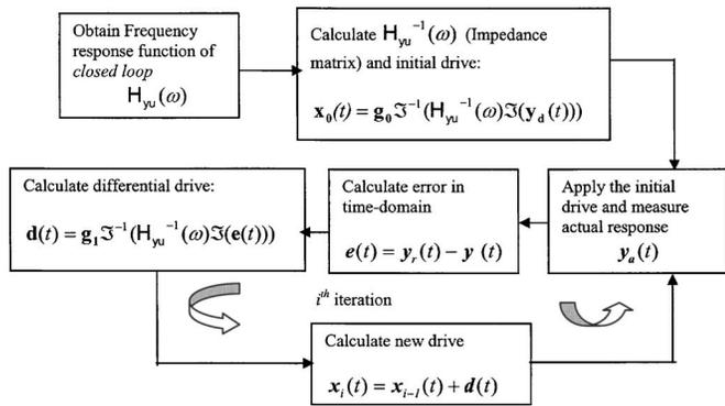
Fig. 3. Iterative scheme for multiactuator control
