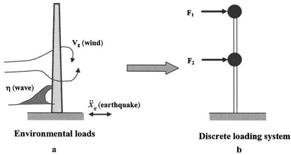
Fig. 8. (a) Environmental loading; (b) discrete loading system
