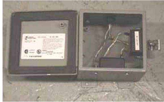
FIGURE 9.3. Columbia accelerometer (left) and accelerometer pair in enclosure ready for mounting
