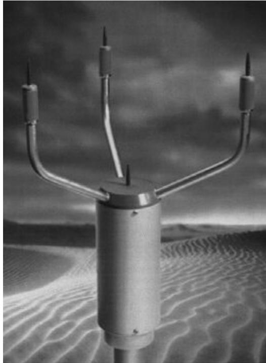
FIGURE 9.7. Photo of Viasala ultrasonic anemometer
