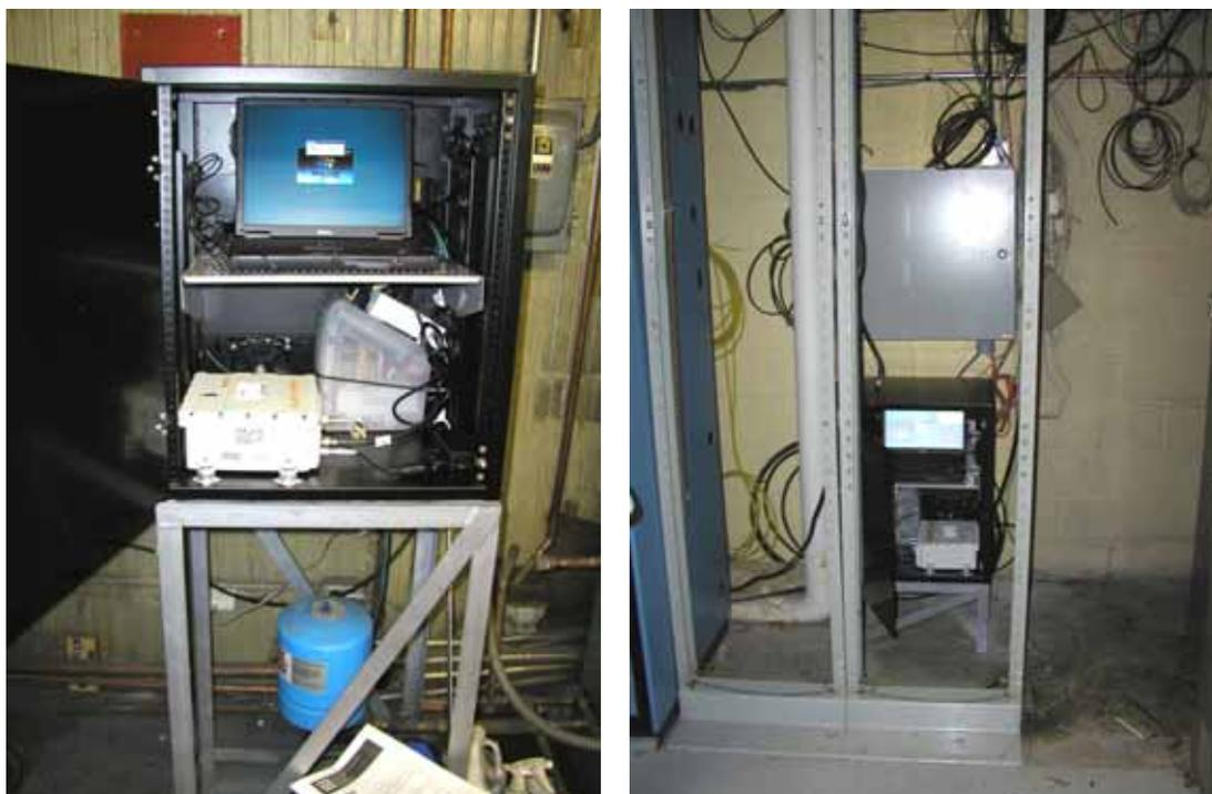
FIGURE 13.6. GPS Instrumentation cabinet in place at reference site (left) and at rover site just below data logger cabinet in Building 1
