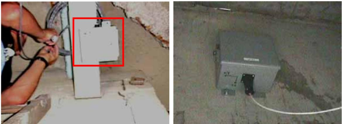
FIGURE 9.6. Mounted accelerometer housing in Building 1 (left) and Building 2
