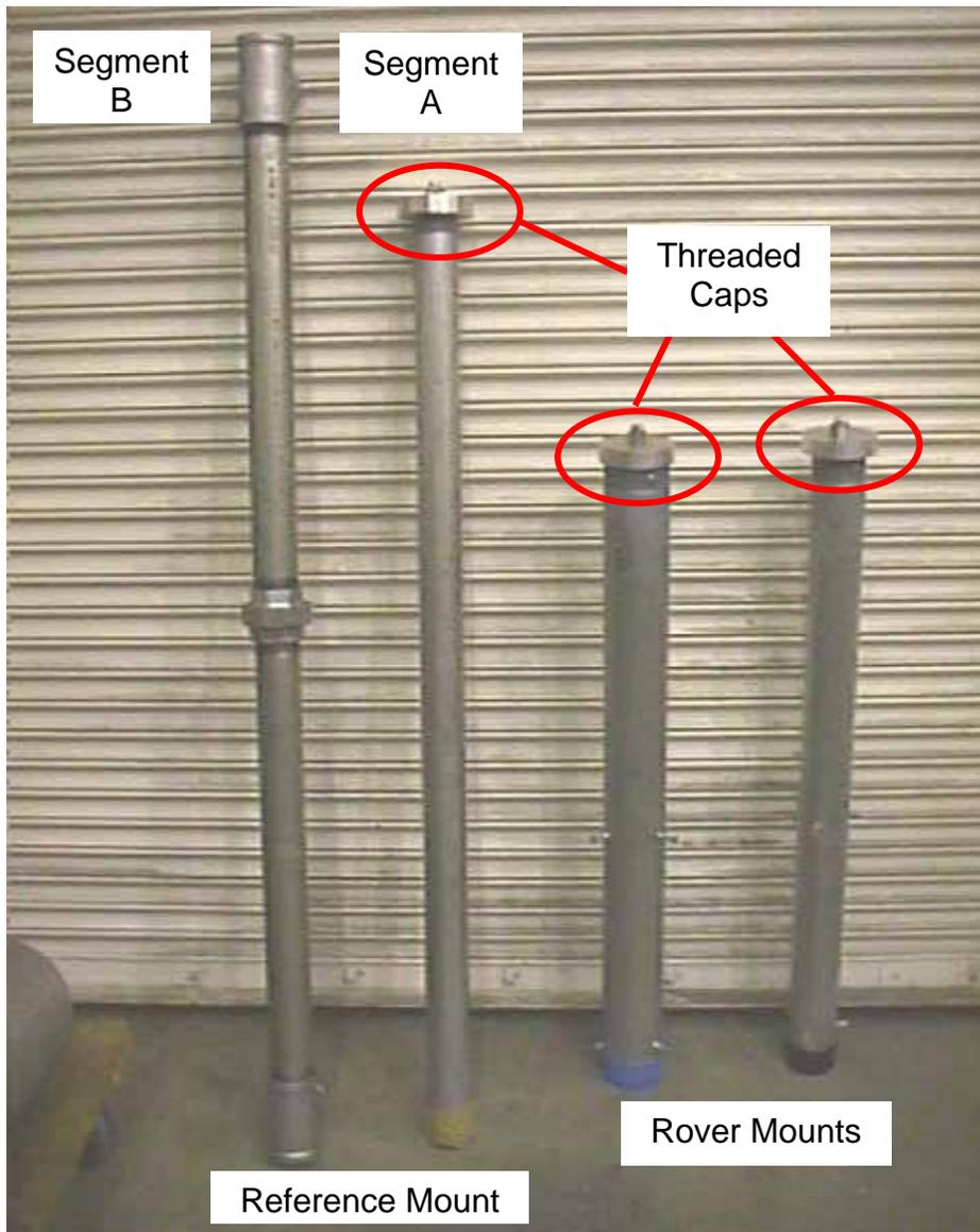
FIGURE 13.1. Reference and rover antenna mounts fabricated for full-scale application
