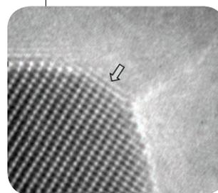
nanowires out of an aluminum droplet. The liquid aluminum brings oxygen to the growing wire surface, in alternating growth and dissolution reactions at the edge of the wire. The oscillation created an optimum face
