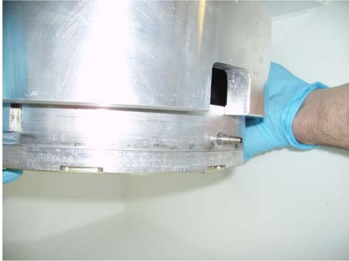
2. When the puck and carrier head are aligned push upwards until the puck contacts with the inside face of the carrier head. Rotate clockwise. When the puck is released it will drop down into a channel and be held securely in a bayonet style attachment.
