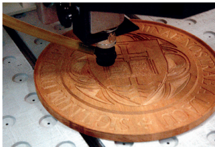
The sign shop created the Notre Dame seal in wood for the tabletop inlays. Cutting the seal took eight hours and five different bits.
