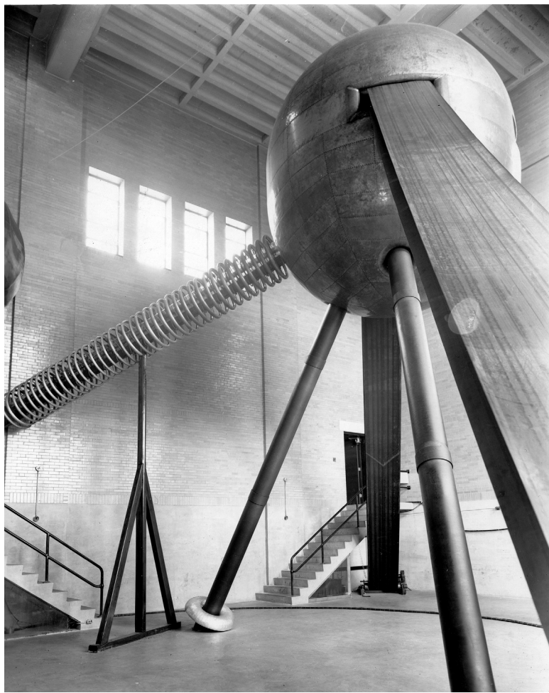
The physics department's Van de Graaff particle accelerator, shown here in a photograph taken around 1935, was then one of the country's first and most powerful particle accelerators. Photo supplied by Elizabeth Hogan, Notre Dame Archives.
