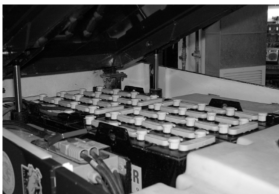
Under the hood, the Zamboni is powered by 40 batteries.
