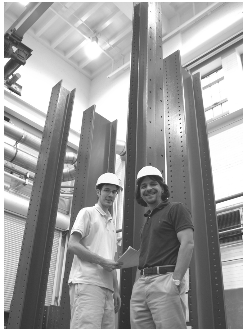
Yahya "Gino" Kurama and graduate student Brian J. Smith discuss progress on a structure they are building to simulate the power of an earthquake on prefabricated walls of Kurama's design. The sample walls will be supported by the girders then assaulted with powerful waves from a hydraulic actuator. ND Works staff photo.
