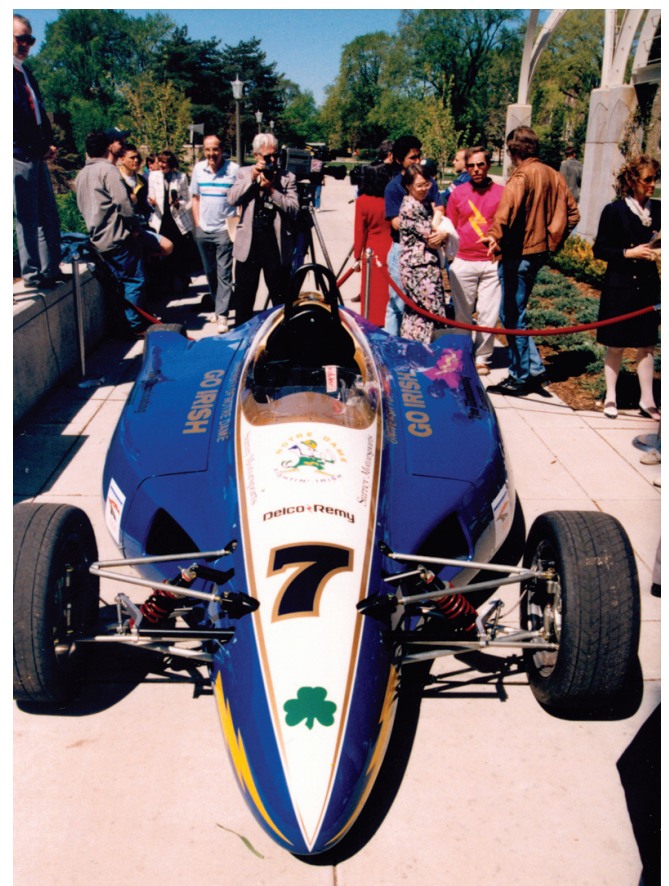
Powered by 12-volt batteries, this open wheel race car hit speeds of 160 miles per hour.
