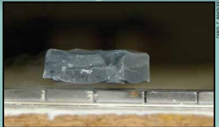
Superconductivity, which plays a central role in the movie "Avatar," is real science, says Morten Eskildsen, associate professor of physics. Above, he shows how a superconducting ceramic material, cooled with liquid nitrogen, will levitate in a powerful magnetic field.
