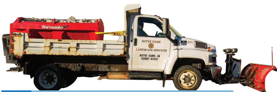
2 1 1/2-Ton Trucks to plow and salt campus roads
