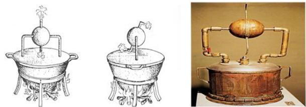
Figure 14. Representations of the steam boiler from Heron's writings and physical reconstruction of the device.
