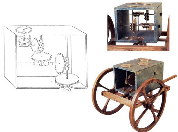
Figure 15. Heron's odometer and reconstructions of the odometer by Woodcraft.
