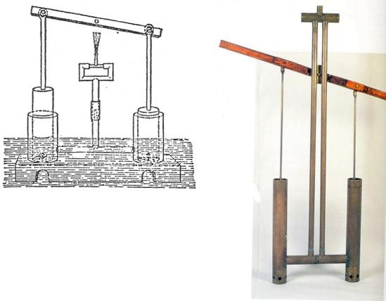
Figure 10. The force pump of Ktesibius and modern reproduction.
