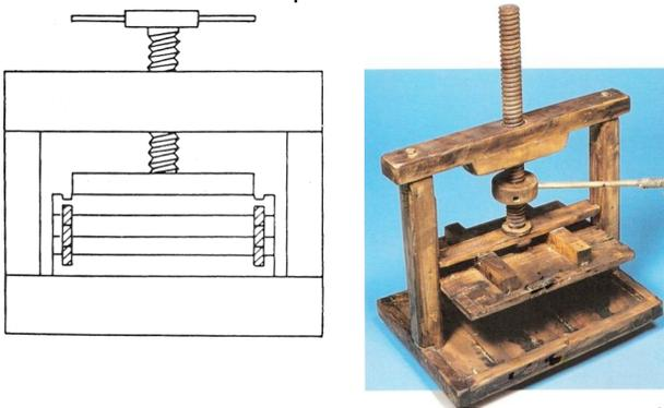
Figure 11. Representation of the oil press and modern reproduction.
