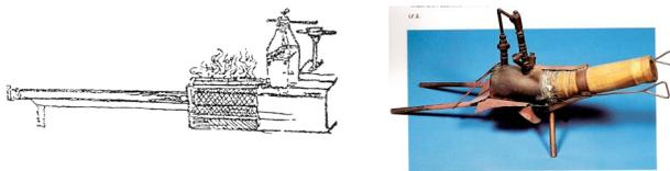
Figure 5. The steam gun invented by Archimedes and its reproduction.
