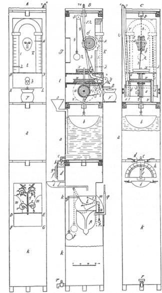
Figure 7. Drawing of the water clock of Archimedes. The façade (A), the cross section (B) and the back view (C).
