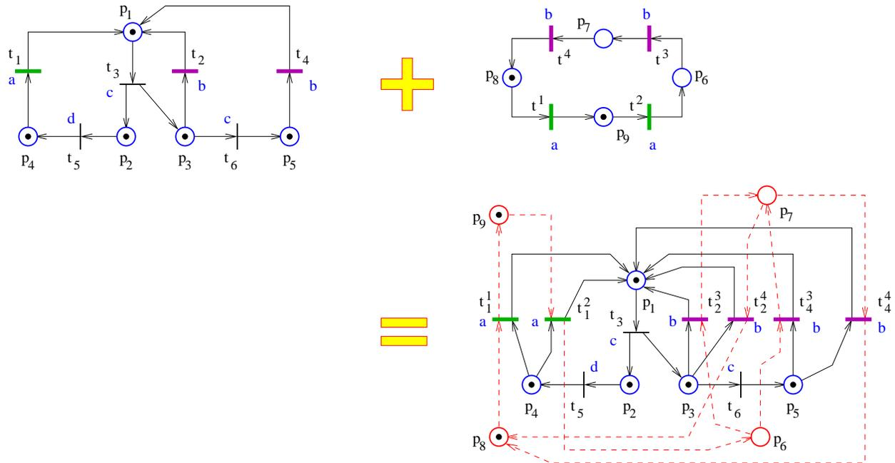
Figure 16: Parallel composition example. The letters  $a$ ,  $b$ ,  $c$ , and  $d$ , denote the labels.
