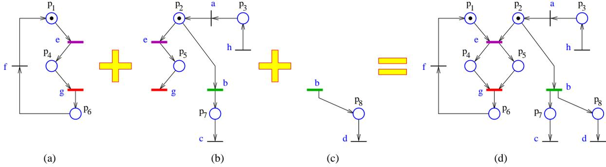
Figure 3: PNs that represent programs are a composition of state machine components. Note that the transitions with the same label are composed.
