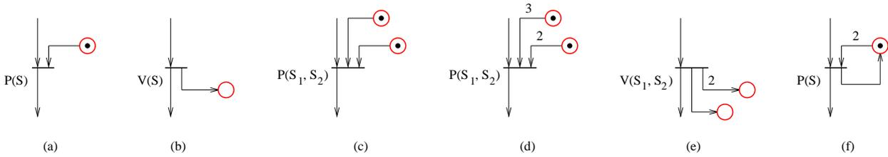
Figure 12: Regular P and V operations represented at (a) and (b). Next, (c) corresponds to a simultaneous P. Simple extensions are necessary for the operations shown at (d–f). Note the integer arc weights.
