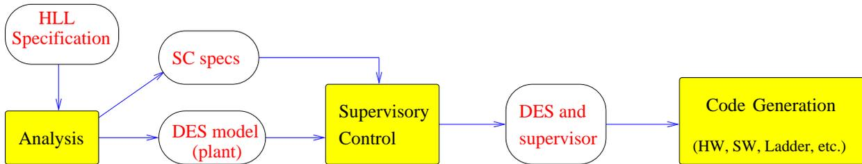
Figure 1: A DES plant and an SC specification are extracted from the user specification. The SC specification describes the objective of the supervision. After the SC tools are applied, the resulting closed-loop DES can be transformed into programming code. While focusing here on program synthesis, the same approach could also be used in other contexts, such as to generate code for hardware implementation or ladder logic for manufacturing applications.
