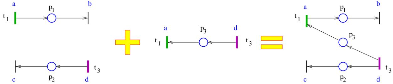
Figure 15: Parallel composition example. The letters  $a$ ,  $b$ ,  $c$ , and  $d$ , denote the labels.
