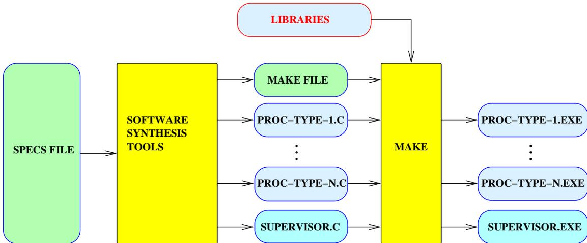
Figure 5: How the software synthesis tools are applied.
