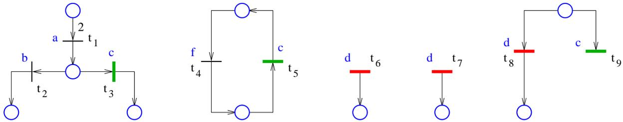
Figure 13: Examples of synchronization and action transitions.  $t_1$  is a synchronization transition since it has an input arc of weight 2.  $t_3$ ,  $t_5$ , and  $t_9$  are also synchronization transitions.  $t_6$ ,  $t_7$ , and  $t_8$  are action transitions.
