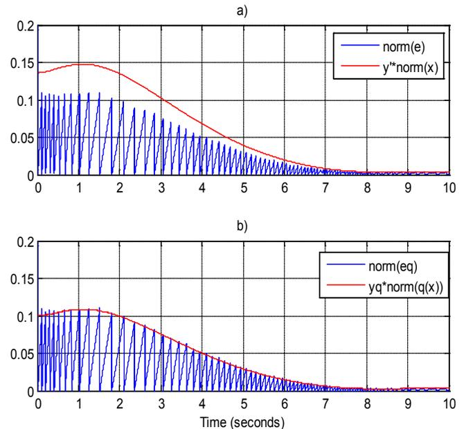
Fig. 5. Response of: a)  $|e(t)|$  and  $y'|x(t)|$ . b)  $|e_q(t)|$  and  $y_q|q(x(t))|$ , for fixed admissible time delay and ZOH model using the same parameters as in example 2.
