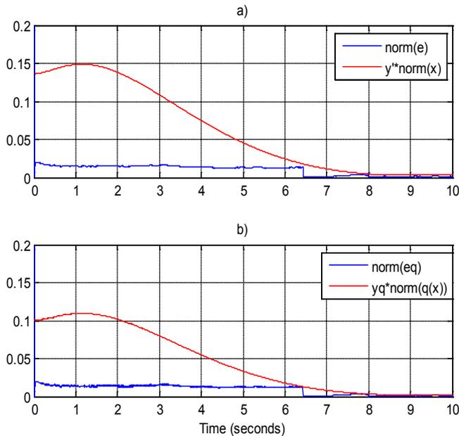
Fig. 4. Response of: a)  $|e(t)|$  and  $y'|x(t)|$ . b)  $|e_q(t)|$  and  $y_q|q(x(t))|$ , for fixed admissible time delay.
