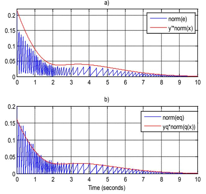
Fig. 7. Response of: a)  $|e(t)|$  and  $y'|x(t)|$ . b)  $|e_q(t)|$  and  $y_q|q(x(t))|$ , for the roll/yaw axes, fixed quantization parameter  $\delta$  and ZOH model using same parameters as in example 3.
