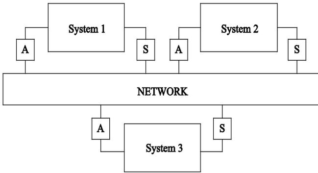
Fig. 1. Representation of Networked Control Systems. A: actuator nodes. S: sensor nodes.
