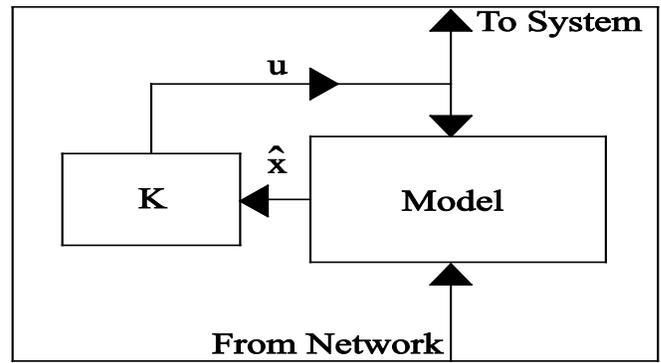
Fig. 2. Model-Based Networked Control System actuator/controller node.
