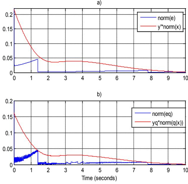
Fig. 6. Response of: a)  $|e(t)|$  and  $y'|x(t)|$ . b)  $|e_q(t)|$  and  $y_q|q(x(t))|$ , for the roll/yaw axes and fixed quantization parameter  $\delta$ .
