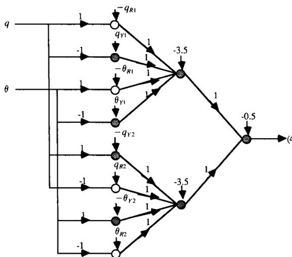
Fig. 12. Numeric/symbolic converter for aircraft fault mode 4.
