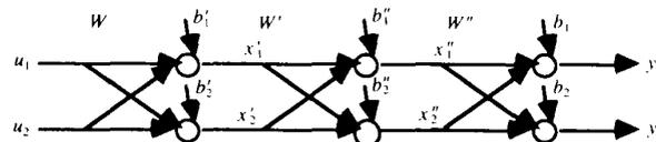
Fig. 2. Multilayer perceptron for two nodes at each layer.
