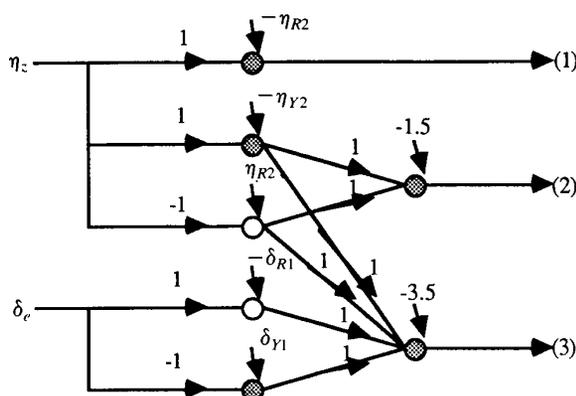
Fig. 10. Numeric/symbolic converter for aircraft fault modes 1-3.
