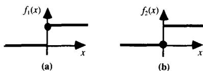
Fig. 3. Threshold nonlinearities for the multilayer perceptron.
