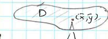
Lamina balances when supported at the center of mass
