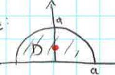
Semicircular lamina  $x^2+y^2 \leq a^2$ , density proportional to the center of the circle,  $\rho(x,y) = K\sqrt{x^2+y^2}$ .
