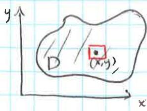
Lamina (plate), density  $\rho(x, y) = \lim \frac{\Delta m}{\Delta A}$  mass in a tiny rectangle about  $(x, y)$
