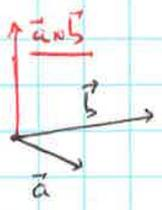
direction of  $\vec{a} \times \vec{b}$  is given by right hand rule.
