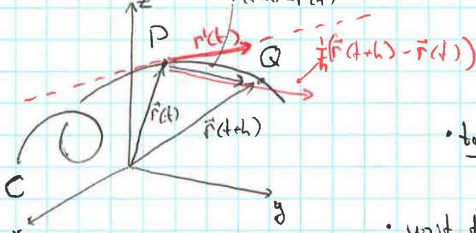
$\vec{r}'(t)$  - tangent vector to curve  $C$  at point  $P$  (if  $\vec{r}'(t) \neq 0$ ) and exists
