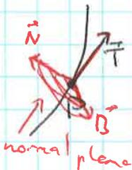
plane through  $\vec{T}, \vec{N}$  - "osculating plane"
