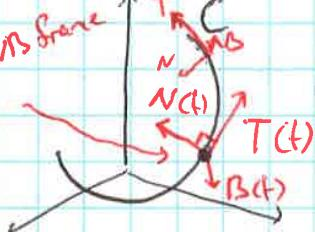
$\vec{B}(t) = \vec{T}(t) \times \vec{N}(t)$  - (unit) binormal vector
