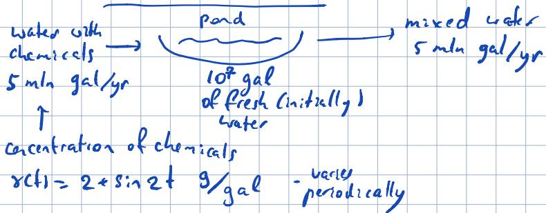
$$\frac{dQ}{dt} = \text{rate in} - \text{rate out} = 5 \cdot 10^6 (2 + \sin 2t) - \frac{Q}{10^7} 5 \cdot 10^6$$
