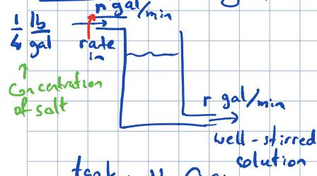
tank with  $Q(t)$  lb of salt dissolved in 100 gal of water.
