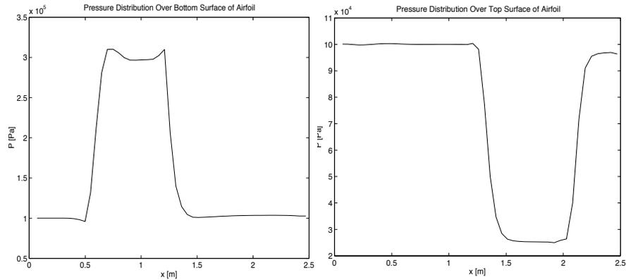
Figure 6: Pressure distribution over both the top and bottom surfaces of a diamond shaped airfoil.
