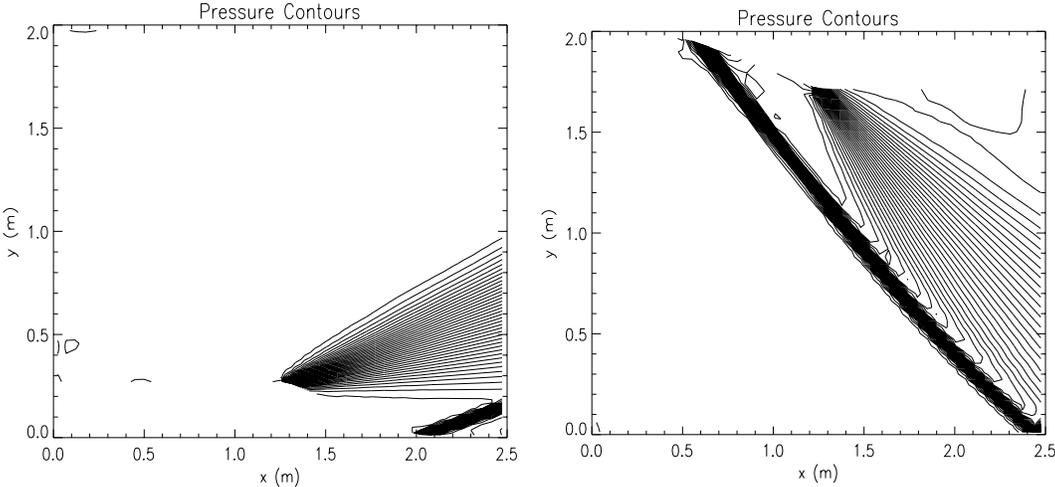
Figure 3: Contour plot of pressure over both the top and bottom surfaces of a diamond shaped airfoil.
