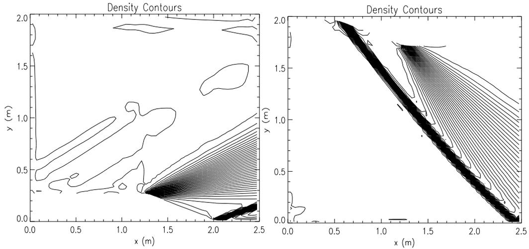
Figure 5: Contour plot of density over both the top and bottom surfaces of a diamond shaped airfoil.
