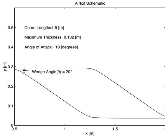
Figure 1: Schematic of diamond shaped airfoil.
