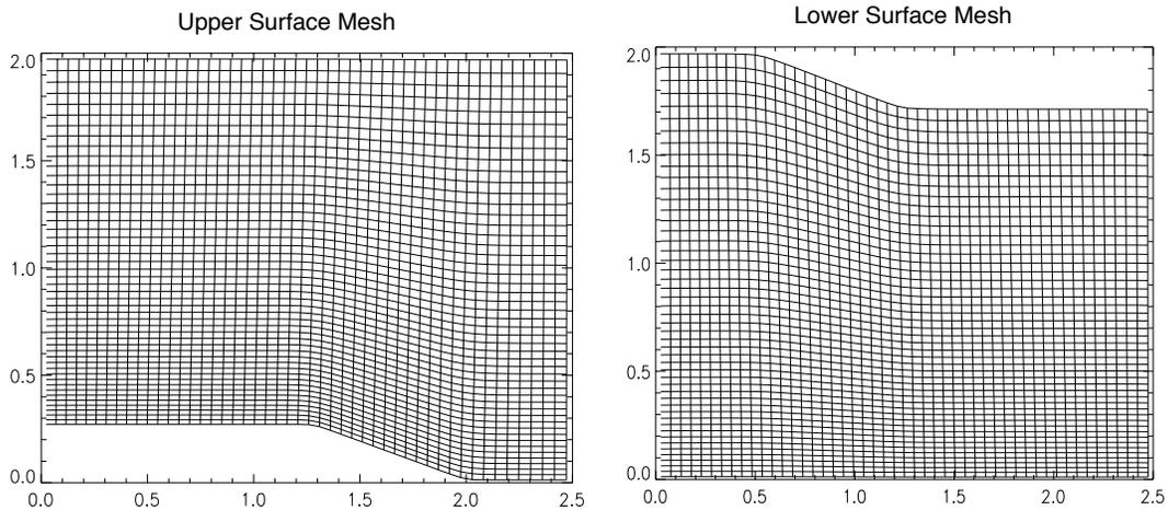
Figure 2: Mesh generated around the diamond shaped airfoil.
