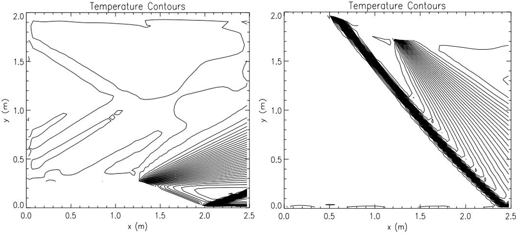
Figure 4: Contour plot of temperature over both the top and bottom surfaces of a diamond shaped airfoil.
