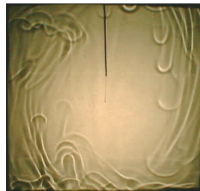
Figure 1. A shadowgraph showing the spatial distribution of thermal plumes in a Rayleigh-Bénard cell. The fluid is dipropylene glycol, which has a rather high viscosity (Prandtl number = 596), so the pattern of plumes appears in a simplified form. The Rayleigh number is 6.8 \times 10^8 . (The picture was taken by S. Lam in Keqing Xia's laboratory and is part of a joint project with Penger Tong.)
