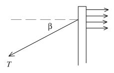
expression for the horizontal component of T. Let T = 20,000 pounds, take  $\beta$  equal to  $40^{\circ}, 30^{\circ}$ , and  $20^{\circ}$ , and compute the magnitude of this horizontal component in each case. Do you think that this force is problematic in the context of the solution of the structural problem?
